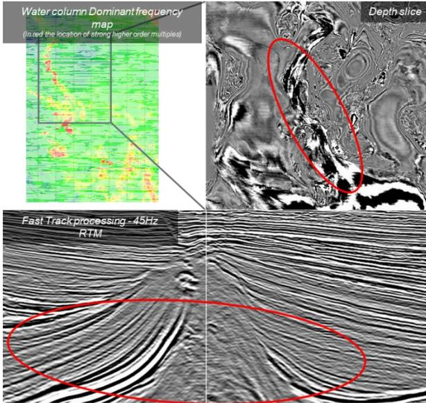
**Figure 4.** Correlation of higher order multiples and geology. Top left image shows the dominant frequency map of the water column. Top right image shows a depth slice around the water bottom. The red circle highlights a canyon on the same location where the higher order multiples are stronger. Bottom image shows the contamination of the higher order multiple on a 45 Hz RTM stack.
