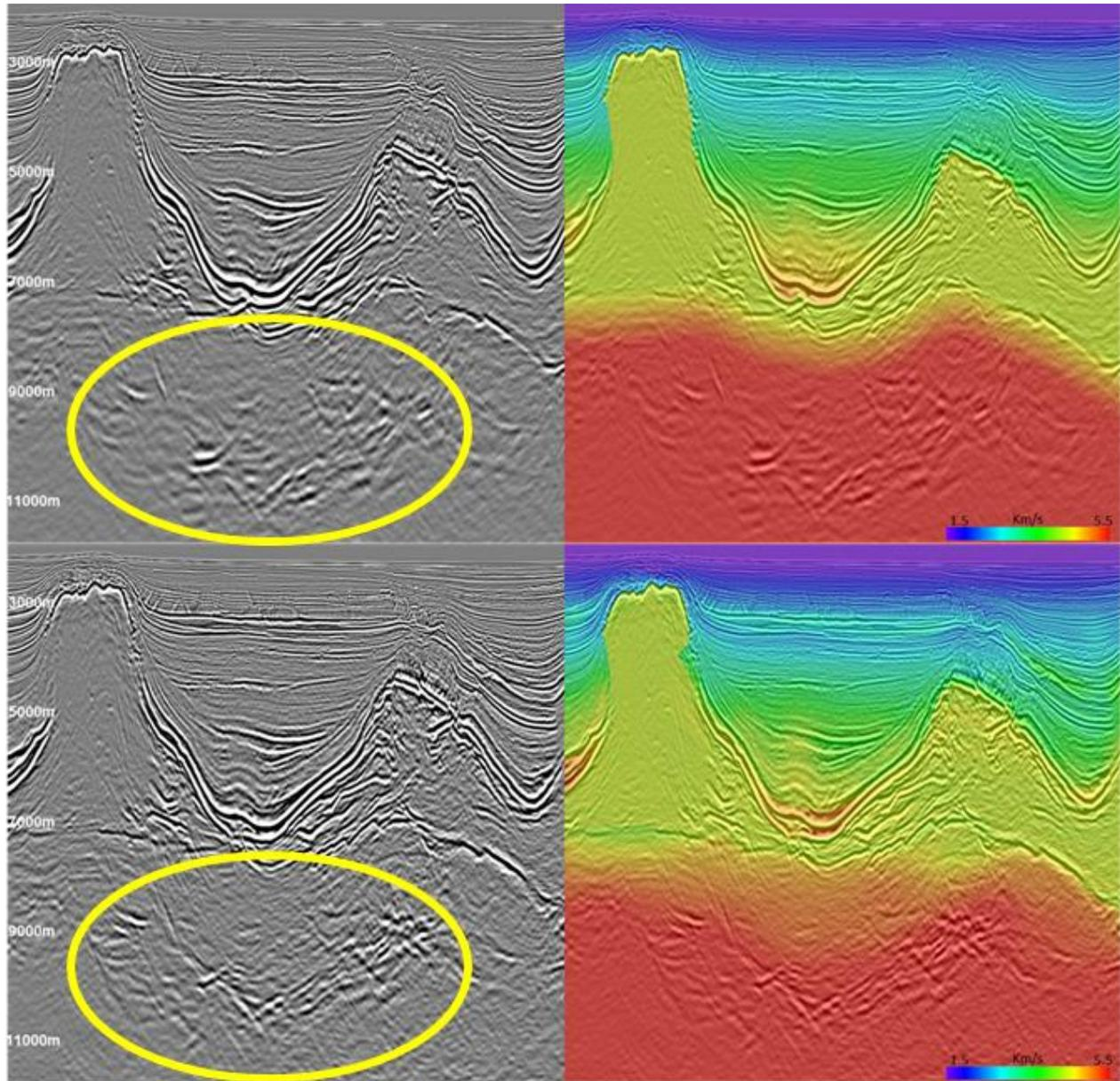
**Figure 8.** Velocity update on pre-salt. Left images show 20 Hz RTM stacks. Right images show 20 Hz RTM stacks overlaid with the velocity models. Top images show the legacy velocity and stack. Bottom images show the updated velocity and stack. Yellow circle highlights the pre-salt events getting more focused and more continuous after the TLFWI update.
