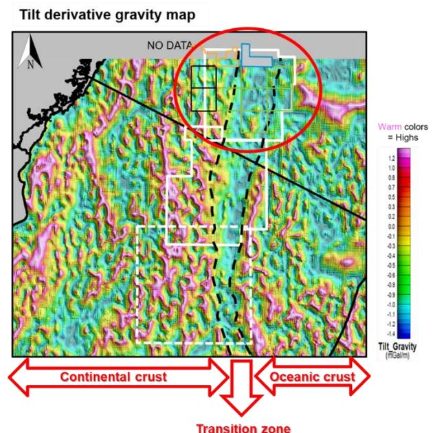
**Figure 1.** Gravity Map of the Espirito Santo Basin. The red circle highlights the survey area. The dashed lines separate the three different domains: West, Central and East.
