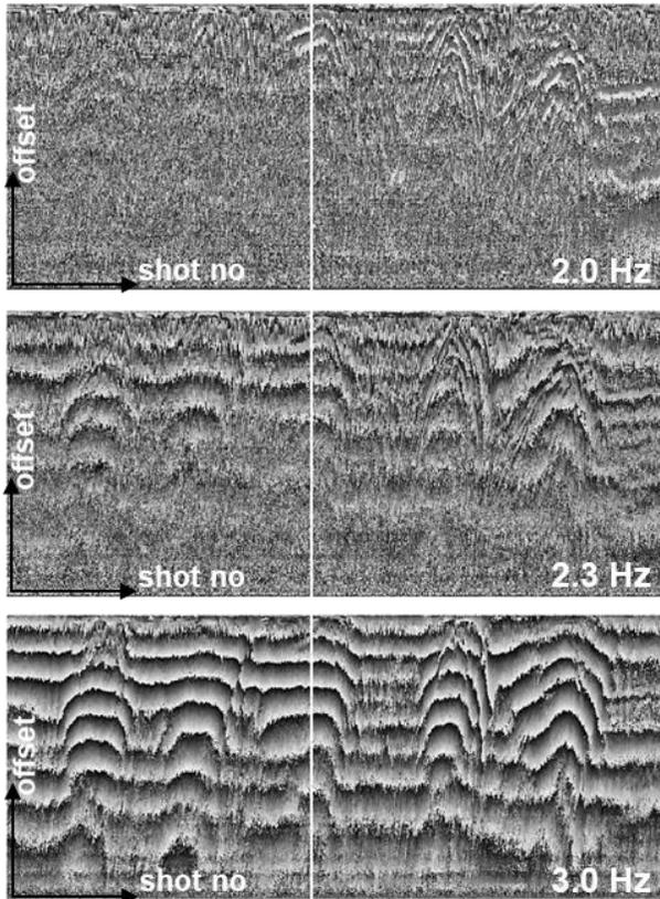
**Figure 2.** Phase QC of data. Top image shows phase QC for 2 Hz, middle image shows phase QC for 2.3 Hz and bottom image shows phase QC for 3.0 Hz. Far offset data shows usable data at 2.3 Hz.
