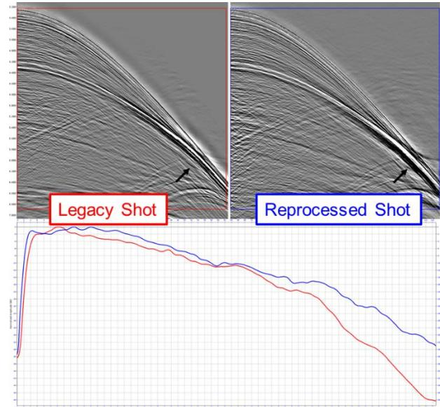
**Figure 3.** Frequency spectra comparison between legacy and reprocessing. Top left image shows a legacy shot. Top right image shows the reprocessing applied to the same shot. Bottom image shows the frequency spectra comparison. The event pointed by the arrow has richer low frequency on the reprocessed shot compared to the legacy shot.
