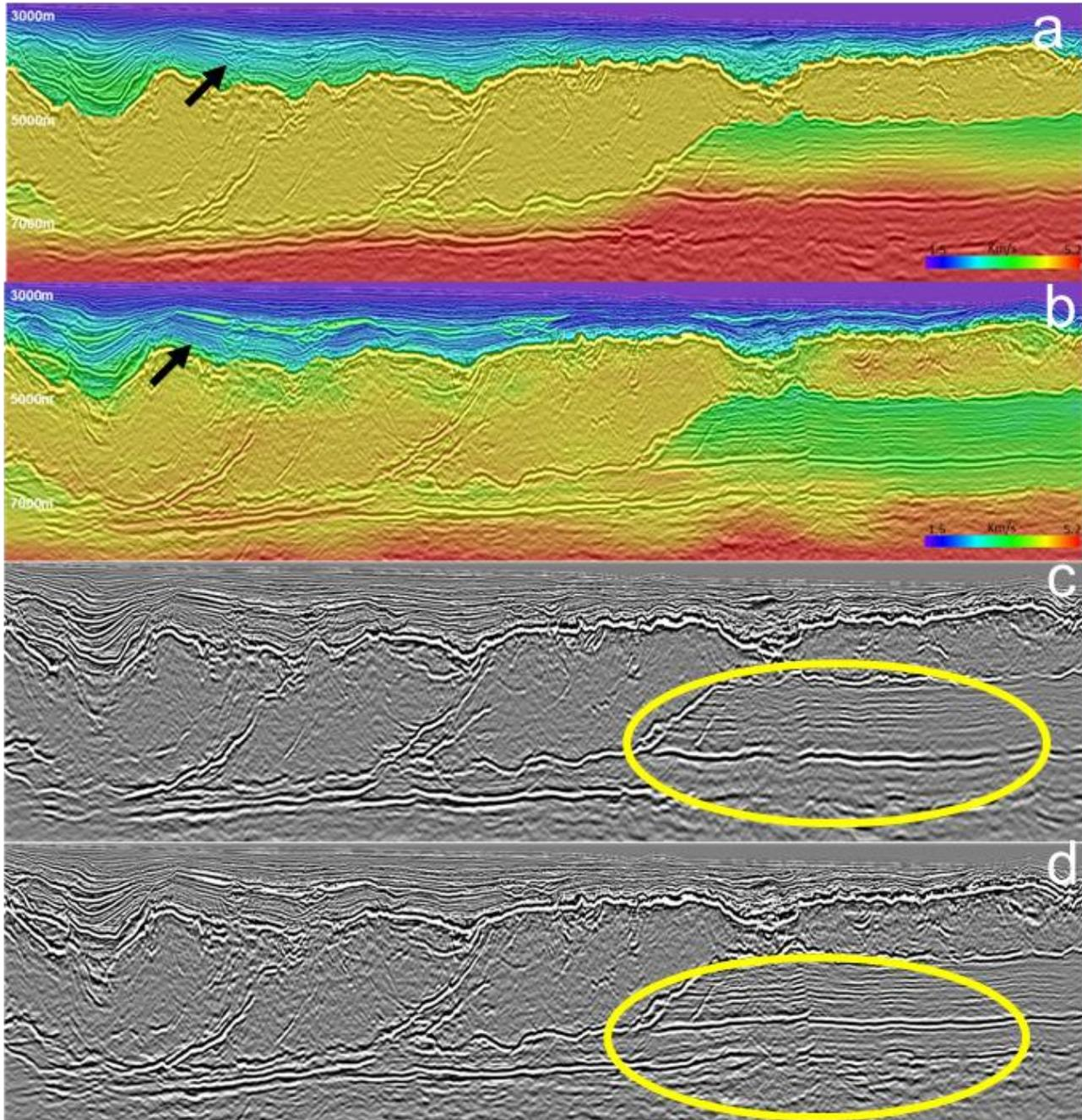
**Figure 7.** Velocity update from the eastern part of the survey. A) Legacy velocity model overlaid on 20 Hz RTM stack. B) Updated velocity model overlaid on 20 Hz RTM stack. C) Legacy 20 Hz RTM stack. D) Updated 20 Hz RTM stack. The yellow circle shows an area where the events are better focused and more continuous after TLFWI update. The arrow shows how the TLFWI can capture better the velocity in the shallow volcanics.
